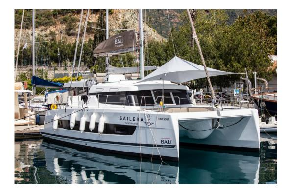
LOA 12,05 m - Beam 6,56 m - Draft 1,10 m Cabins 4, Berths 8+2, Heads 4 Water Tank 700 Lt - Fuel 400 Lt Engine 2x40 HP Yanmar
